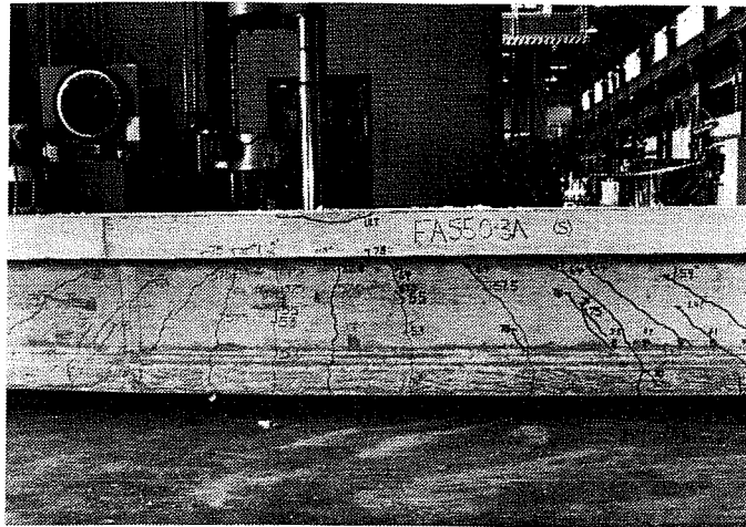
Figure 4.10 Test FA550-3A, Typical Flexural Cracking
